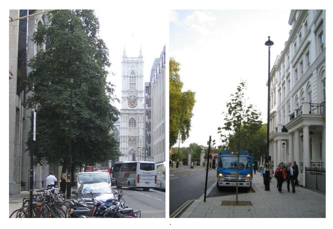
Lighting column with bracket adjacent to tree, the canopy having grown out across the street thus blocking off light to the footway and road past the tree.
