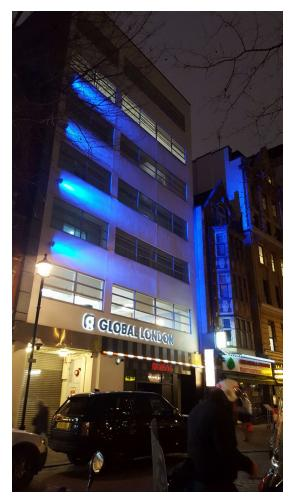
Poor lighting design with excessive spill light
